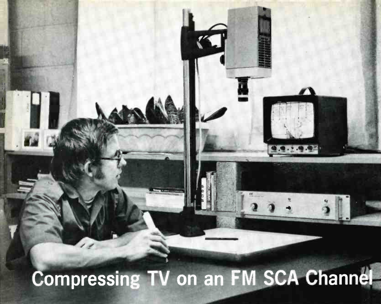
Transmitting terminal can be as simple as a small industrial TV camera, monitor, and video compressor. Location can be up to 10 miles from the transmitter.
